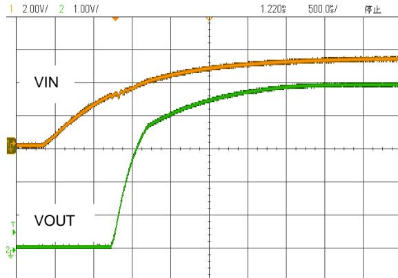
图 23. 软启动,  $V_{IN} = 5.3V$ ,  $V_{OUT} = 5.0V$ ,  $I_o = 3A$
