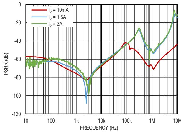
图 19. PSRR,  $V_{IN} = 1.1V$ ,  $V_{OUT} = 0.8V$ ,  $V_{BIAS} = 5.0V$
