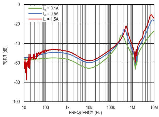
图 20. PSRR,  $V_{IN} = 5.3V$ ,  $V_{OUT} = 5.0V$
