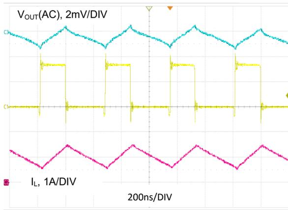
图 23.  $V_{OUT} = 1.2V$ ,  $I_O = 1A$ , FPWM
