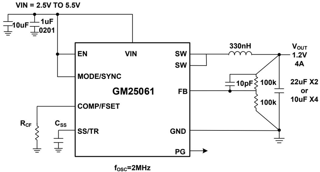
图 34. 2MHz, V<sub>IN</sub>=3.3V, V<sub>OUT</sub>=1.2V, I<sub>LOAD</sub>=4A
