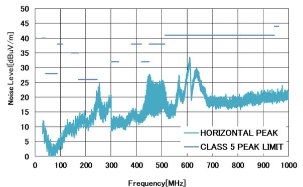
图 32. GM2506\_DEMOZ CISPR25 Radiated Emission (Horizontal)
